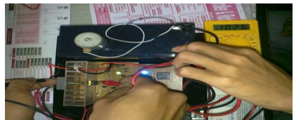
Gambar_7. Rangkaian Battery Charger
