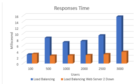
Gambar 9. Grafik Responses time perbandingan load balancing dan load balancing web server 2 down
