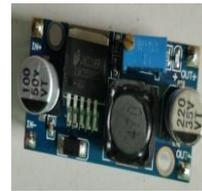
Gambar 2.11 DC Voltage Step-Down
