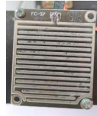
**Gambar 2.3** Rain drop sensor (sensor hujan)
