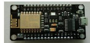
Gambar 2.1 NodeMCU ESP8266
