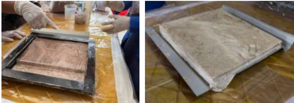
Gambar 6. Proses pencetakan panel atap coco-composite
