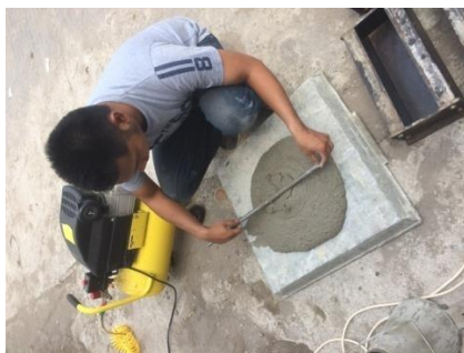
Gambar. 2. Pengujian Slump Flow
