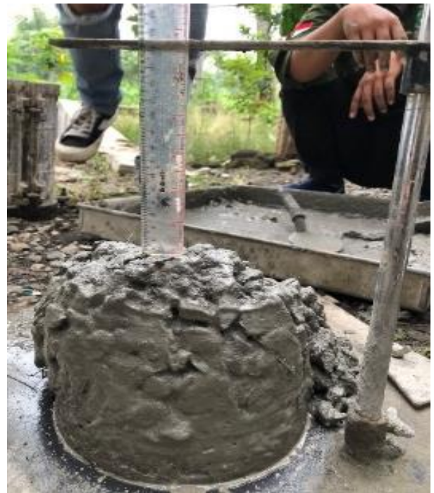
Gambar 2. Uji Slump Beton
